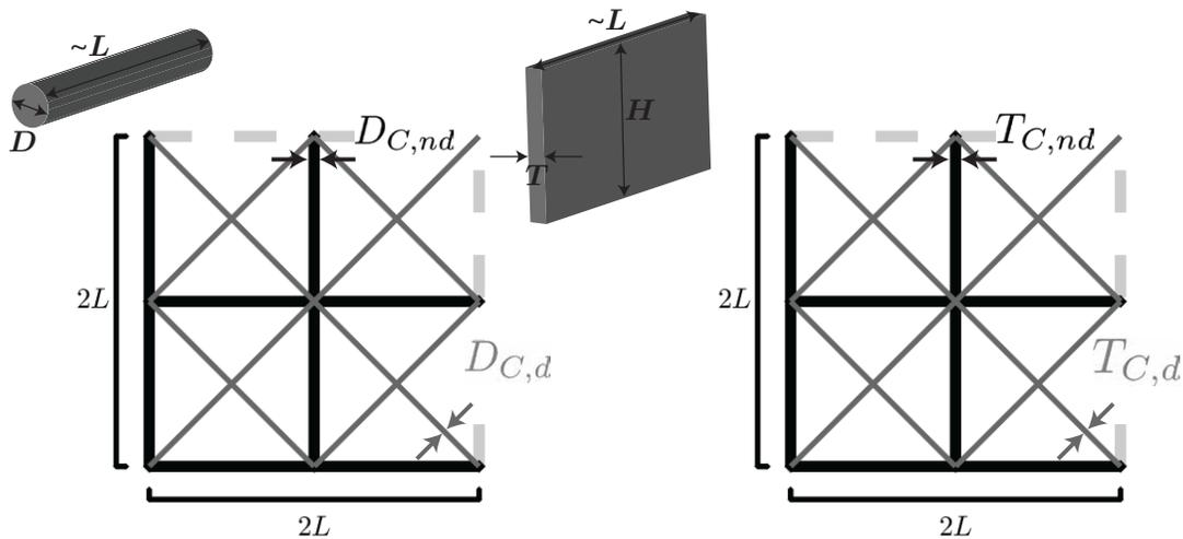
**Supplementary Figure 4:** Unit cell for *Design C*. Schematics of the unit cell for *Design C* (all cells filled with diagonal bracings, as is typically found in infrastructure applications). On the left we indicate the geometric parameters of this design considering a circular cross-section, while on the right we show the geometric parameters of this design considering a rectangular cross-section.
