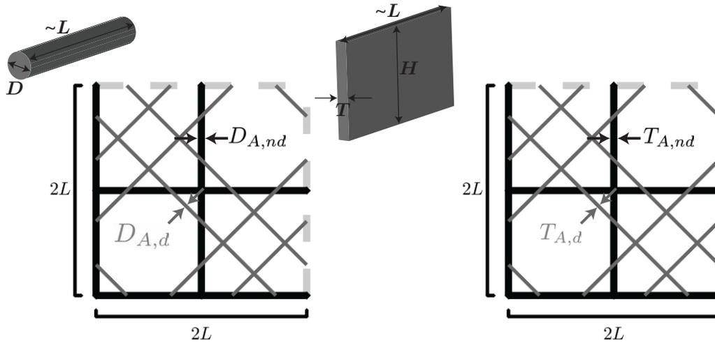
**Supplementary Figure 2:** Unit cell for *Design A*. Schematics of the unit cell for *Design A* (the sponge-inspired lattice). On the left, we indicate the geometric parameters of this design considering a circular cross-section, while on the right, we show the geometric parameters of this design considering a rectangular cross-section.
