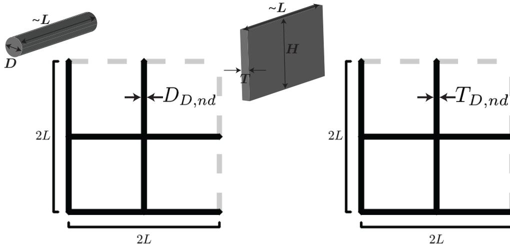
**Supplementary Figure 5:** Unit cell for *Design D*. Schematics of the unit cell for *Design D* (square lattice with no diagonal reinforcement). On the left we indicate the geometric parameters of this design considering a circular cross-section, while on the right we show the geometric parameters of this design considering a rectangular cross-section.
