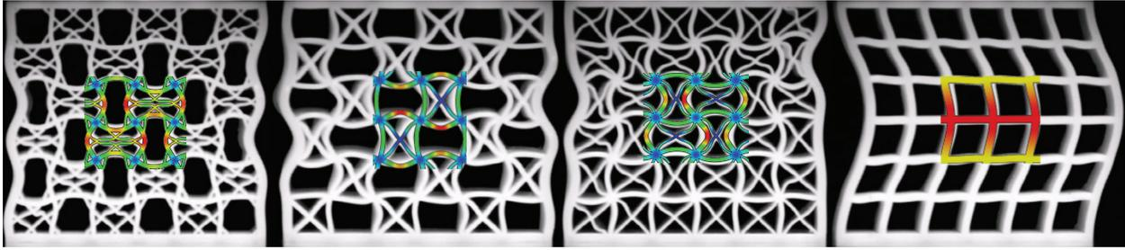
**Supplementary Figure 13: Comparison between experimental and numerical results.** This figure shows experimental snapshots of the experimental specimens at an applied 8% compressive strain overlaid with a cutout of the representative deformation predicted by our FE analyses. The close agreement between the experiments and simulations suggests that the FE simulations are accurately capturing the physical deformation of the specimens.
