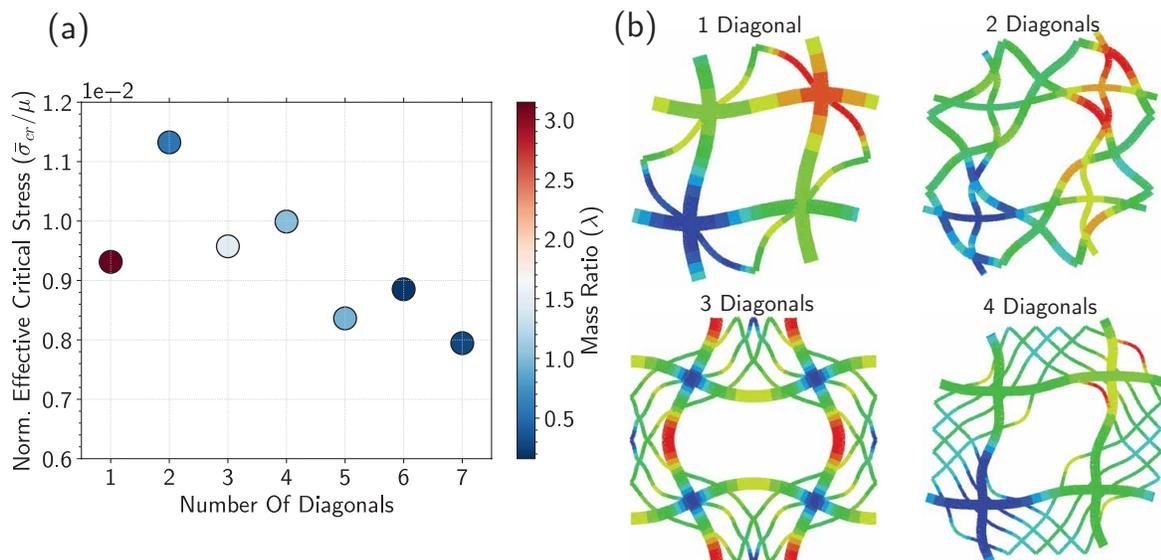
**Supplementary Figure 27: Optimization analysis for infinite periodic structures.** (a) Optimal value of critical buckling stress for varying number of diagonals. The color of each point represents the optimal mass ratio  $\lambda$ . (b) Optimal deformed geometries for designs including one to four diagonals. The color in each structure represents the magnitude of the displacement.
