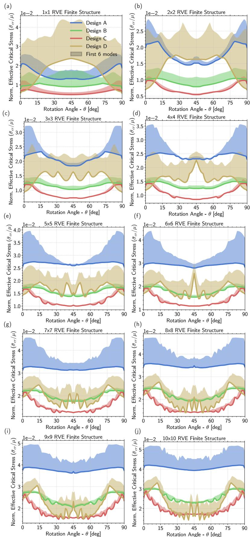
**Supplementary Figure 20: Effect of sample size on critical stress.** Evolution of the effective buckling stress as a function of the loading angle  $\theta$  for finite-size lattice structures comprising  $M$  by  $M$  unit cells, where  $M$  ranges from (a) 1 to (j) 10. The shaded parts in (a) - (j) represent the lowest six buckling modes range. All plots provide a clear indication on the superior performance of *Design A* when comparing to *Designs C-D*, when  $M > 2$ .
