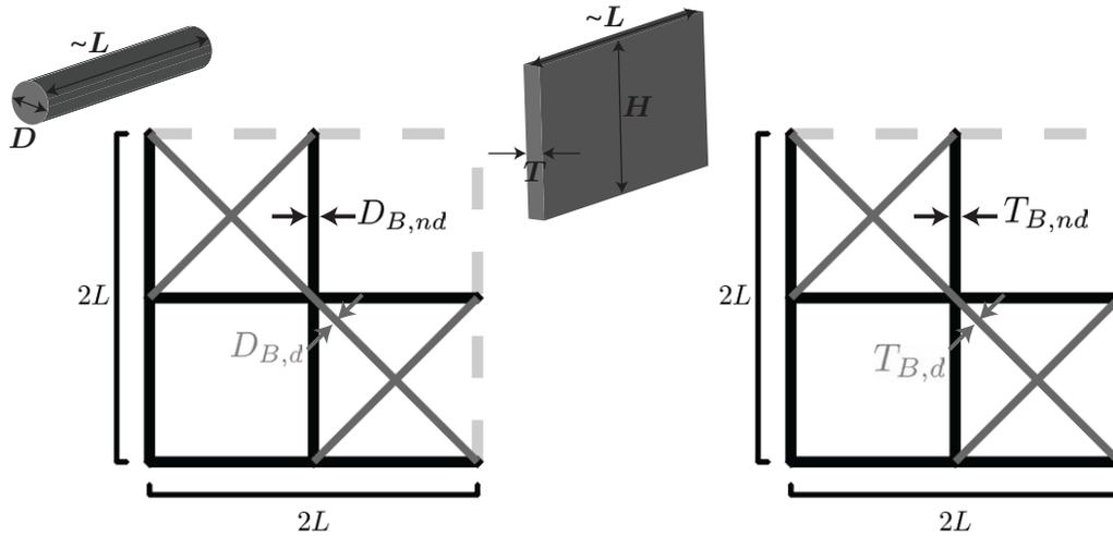
**Supplementary Figure 3:** Unit cell for *Design B*. Schematics of the unit cell for *Design B* (an alternating open and closed cell structure resembling the sponge and employing a single set of diagonal bracings). On the left we indicate the geometric parameters of this design considering a circular cross-section, while on the right we show the geometric parameters of this design considering a rectangular cross-section.
