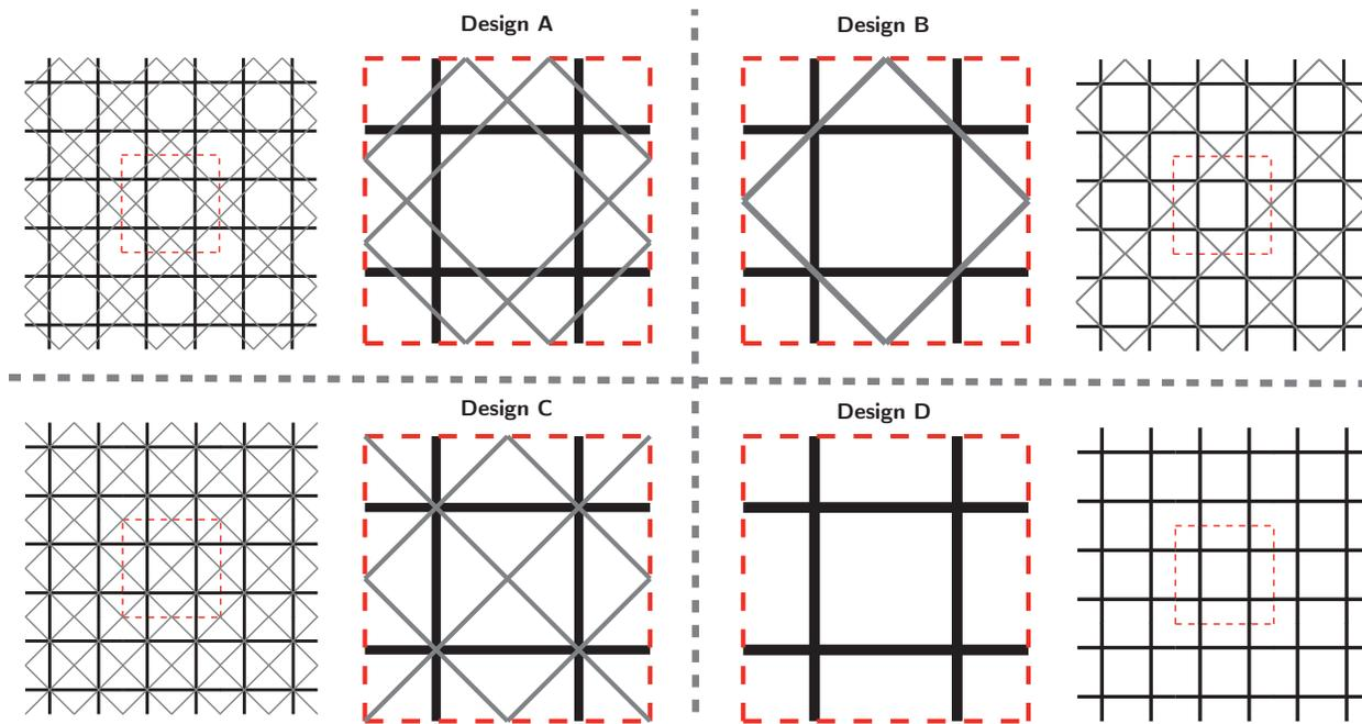
**Supplementary Figure 6: RVE used for the different designs.** Schematics of the RVEs used for *Design A-D*. Periodic boundary conditions are applied on the nodes that intersect with the red dashed line.
