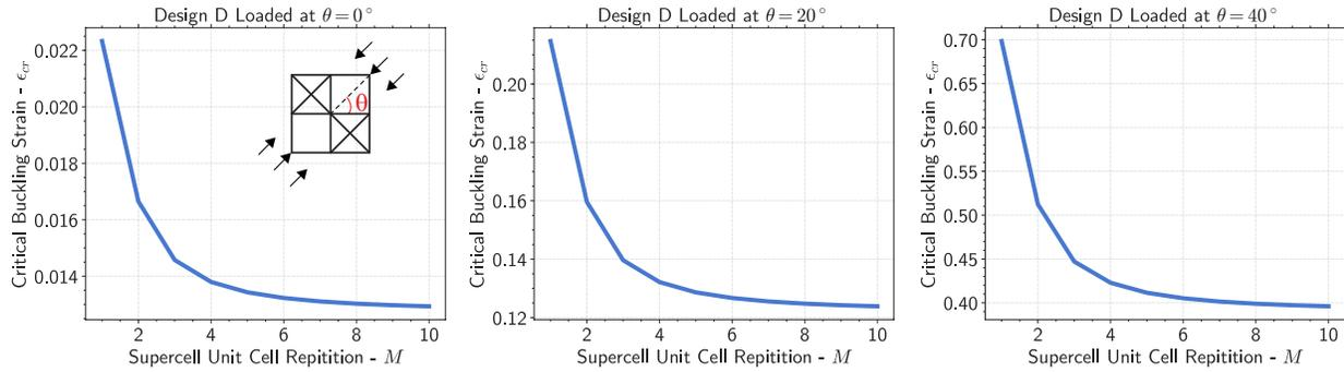
**Supplementary Figure 8:** Critical strain for *Design D* at three selected loading angles. As the number of minimum RVEs  $M$  considered increases, the value for the critical buckling strain asymptotically approaches a constant.
