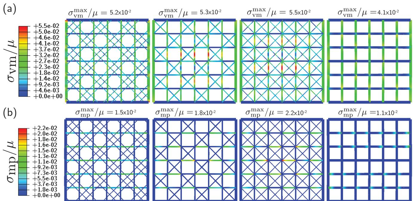
**Supplementary Figure 22: Stress Analysis.** Numerical snapshots extracted from non-linear FE analysis (with first mode imposed imperfection) at an imposed strain  $\epsilon = 0.001$ . (a) The color indicates the normalized von Mises stress  $\sigma_{vm}$  with the maximum value for each structure indicated above each figure. (b) The color indicates the normalized maximum principle stress  $\sigma_{mp}$  with the maximum value for each structure indicated above each figure.
