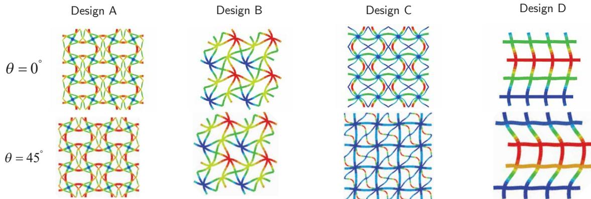
**Supplementary Figure 17: Critical modes of Design A-D at  $\theta = 0^\circ$  and  $\theta = 45^\circ$ .** These critical buckling modes were calculated using a 10 by 10 super-cell and the snapshots shown here are the center 2x2 cells of the full 10x10 model. Designs A-B in this figure exhibit a similar deformation pattern when loaded at  $0^\circ$  or  $45^\circ$ . However, for Design C-D, different buckling patterns are triggered when loaded at  $0^\circ$  and  $45^\circ$ .
