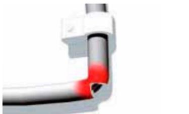
Figure 9: Too tight a bending radius
