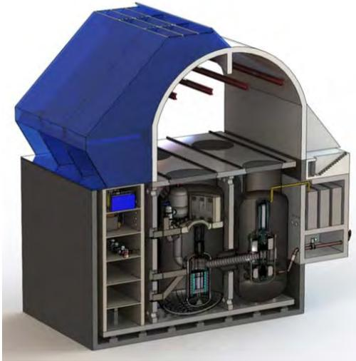
Elevation view of EM<sup>2</sup> modular building element employing two modules on a single seismically isolated platform
