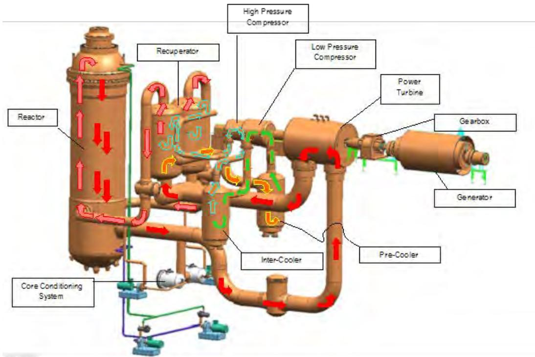
PBMR®-400 power conversion unit components and layout, and He flow.
