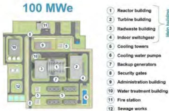
Small NPP layout is sectioned in two areas:
