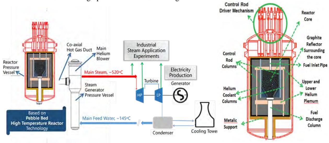
RDE Schematic system (left) and main component of the RPV Internals.
