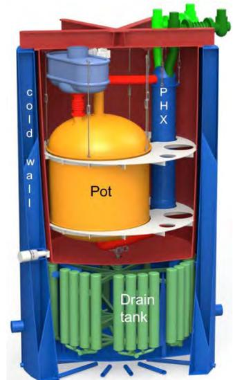
The silo cold wall also cools the Fuel salt Drain Tank (FDT). The drain tank is a circle of (green) vertical tanks to contain hot fuel salt drained from the Pot. This provides sufficient radiating area to keep the peak tank temperature after a drain within the limits of the tank material. This cooling process is totally passive, requiring neither operator intervention nor any outside power.
