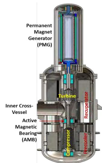
Power conversion unit and generator cutaway
