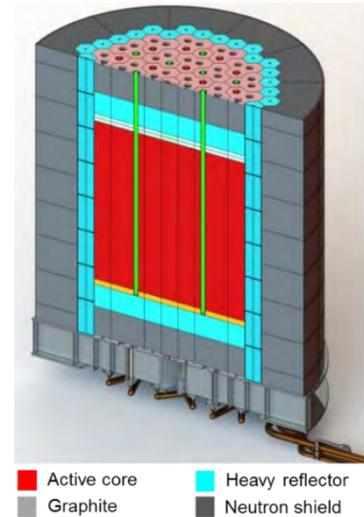
EM<sup>2</sup> core arrangement composed of fuel and reflector.
