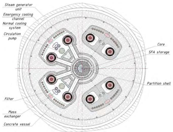
**(a) Engineered Safety System Approach and Configuration**
