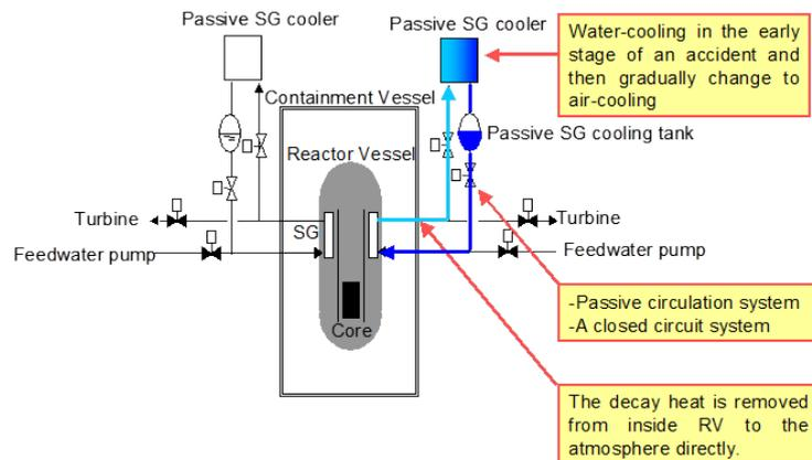
**(a) Engineered Safety System Approach and Configuration**
