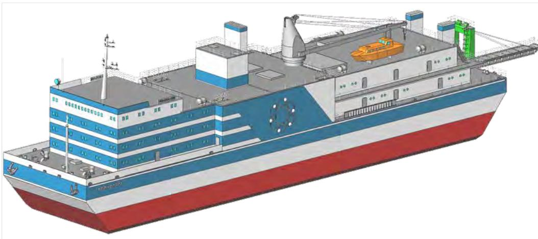
FPU includes reactor, steam-turbine, part of electric power system and control systems. The RPV operates under conditions of 16.2 MPa in the reactor pressure vessel. The steam generators located inside the RPV generate 295°C steam at 3.83 MPa flowing at 55 t/h. The RPV head is located under biological shielding and the control rod drive mechanism is located above the shield outside the vessel.
