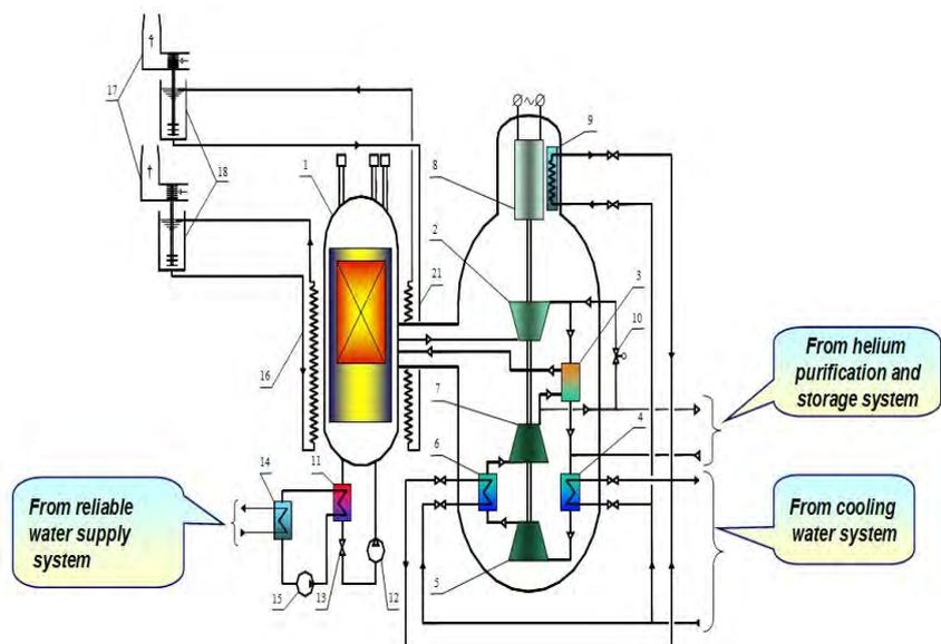
The Brayton power conversion with direct gas turbine contains a gas turbine, an electric generator and gas compressors. The GT-MHR gas turbine power conversion system has been made possible by utilizing large, active magnetic bearings, compact, highly effective gas to gas heat exchangers and high strength, high temperature steel alloy vessels.
