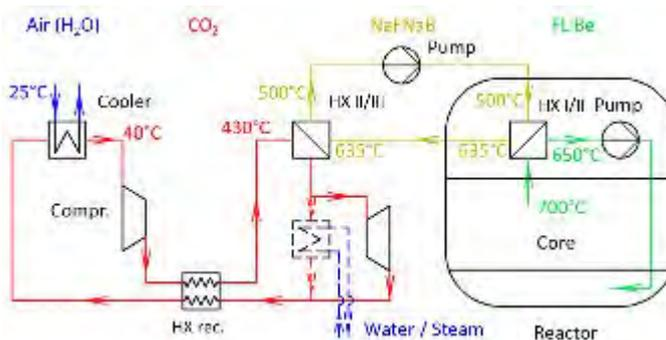
Process Flow Diagram of Energy Well reactor with simple heat recovery system
