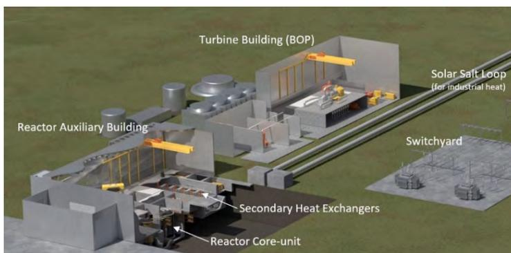
The secondary (non-radioactive) coolant salt lines transfer heat from the operating core-unit primary heat exchangers to secondary heat exchangers and a third, nitrate salt loop located in the nuclear island. The nitrate salt loop transfers the heat from the nuclear island to either steam generators and re-heaters located in the Balance of Plant or directly to an industrial heat end user which could be located up to 5 km from the nuclear island.
