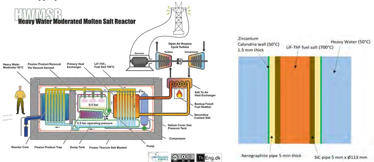
Schematic drawing of a heavy water moderated molten salt reactor (left) and possible core fuel channel insulation configuration (right).
