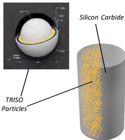
**Fully Ceramic Micro-encapsulated (FCM™) fuel**
