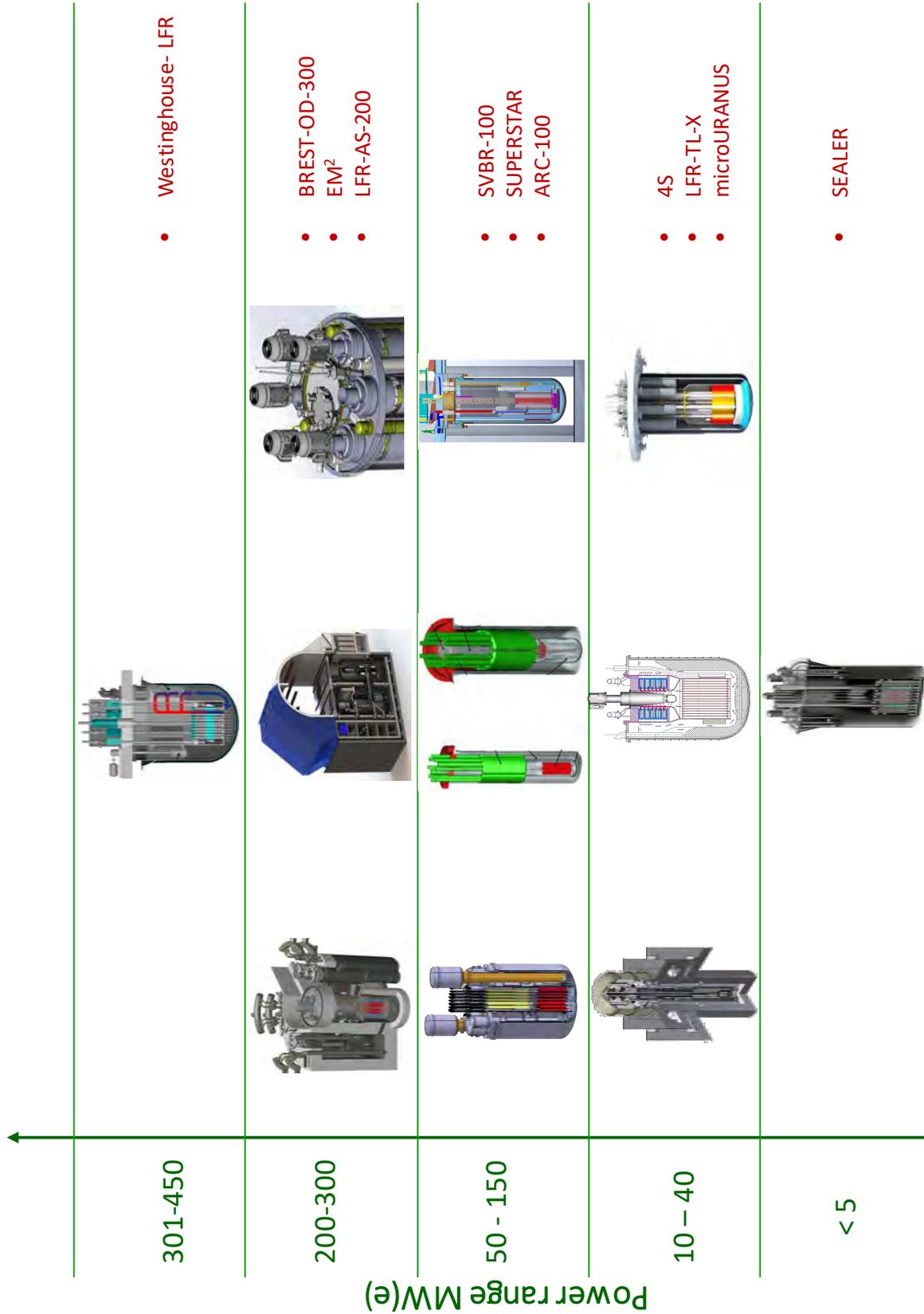
Figure II-4 Power Range of Fast Neutron Spectrum-SMRs
