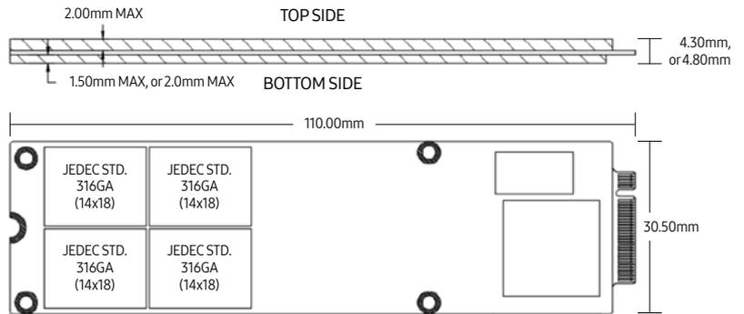
Figure 1 - NGSFF SSD Mechanical Dimensions
