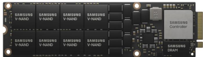
Figure 2 - NGSFF SSD (30.5x110mm) Mounting Two Rows of Eight NANDs (Using Both Sides of PCB, a Total of 16 NANDs Are Mounted)
