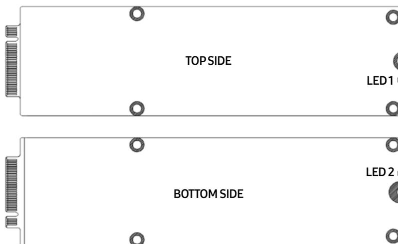
Figure 8: LED Locations on NGSFF Form Factor
