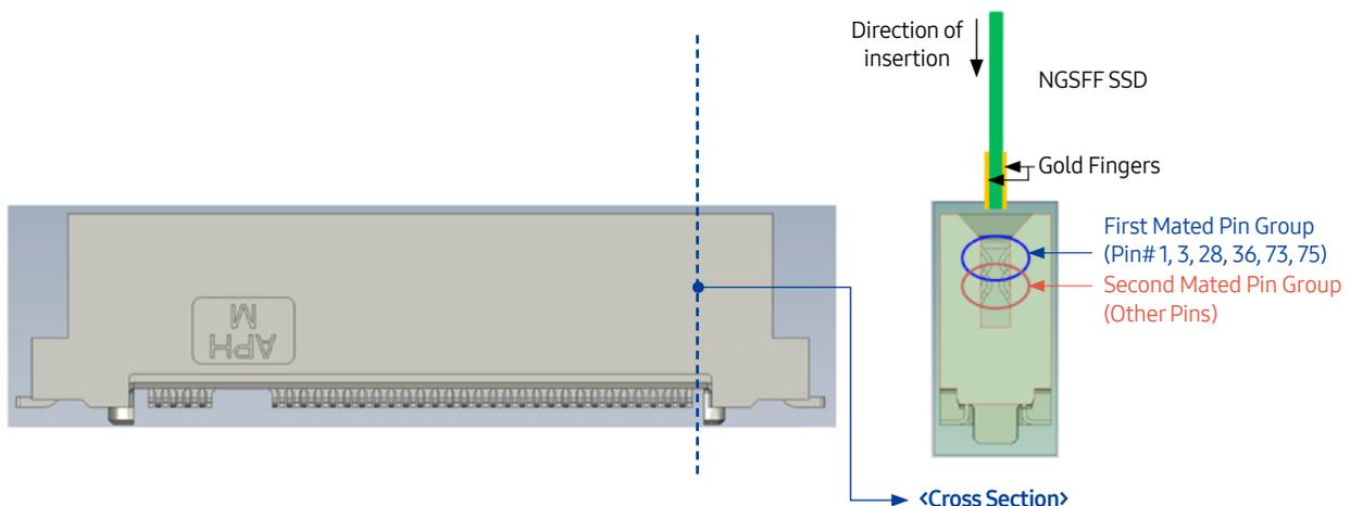
Figure 7: An Example of a Staggered Socket Contact Arrangement for 1<sup>st</sup> Mating Pins to Be Connected First (Cross-Section Drawing of NGSFF SSD Connector)
