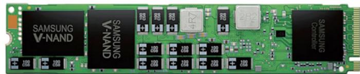
Figure 3 - M.2 SSD (22x110mm) Mounting Only One Row of Two NANDs (Using Both Sides of PCB, a Maximum 4 NANDs Are Mounted)
