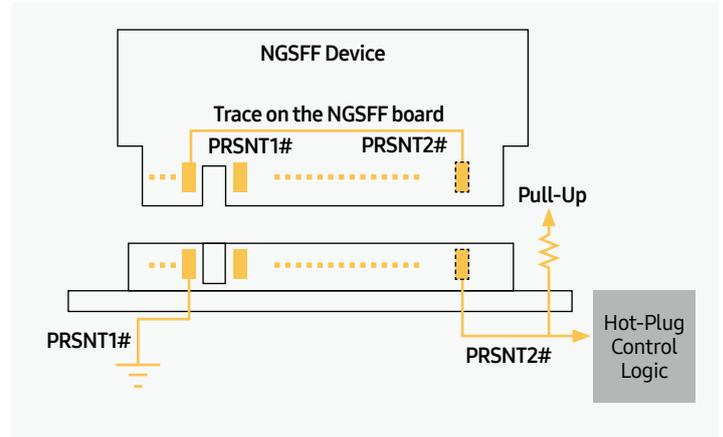
Figure 6: An Example of Host-Side Implementation for Hot-Plug Support Using PRSENT1#/#2
