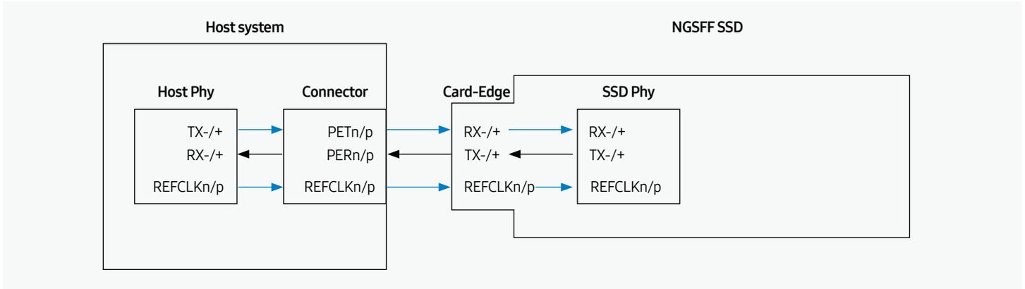
Figure 9: NGSFF SSD Signal Naming Conventions
