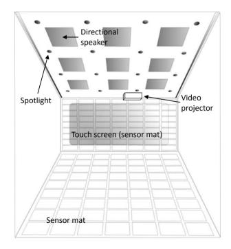
A pilot version of the proactive space with dimensions of  $3 \text{ m} \times 4 \text{ m}$  was constructed at the Aalto University School of Art and Design in Helsinki, Finland. The ELSI (Electric Sensors with Intelligence) research monitoring system by Marimils Ltd. (Tuusula, Finland), based on capacitive sensing, was used for movement detection. The system is capable of simultaneously detecting the
