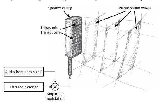
Figure 6. Conceptual drawing and block diagram of an ultrasonic speaker.
