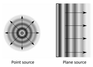
Figure 2. Radiation patterns of theoretical sound emitters.
