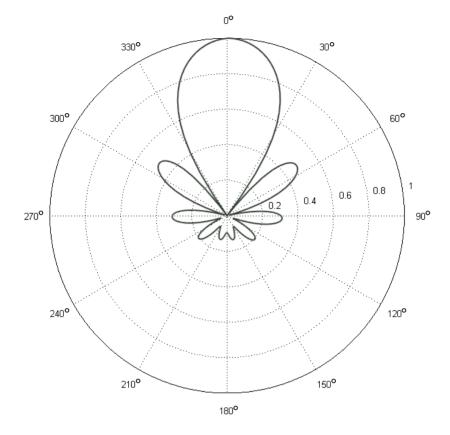
**Figure 5.** Rough conceptual drawing of the directivity pattern of an ultrasonic speaker element. The beam sizes present the proportion of sound emitted in different directions.
