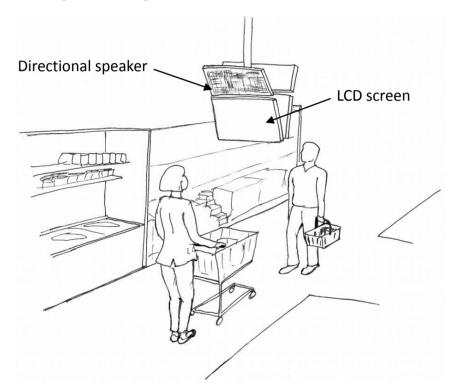
A similar combination of LCD screens and directional speakers is used in the Kamppi shopping mall, Helsinki, Finland. The information stations enable local advertisement without overlapping sound and a marked rise in the noise level. The constant sound strength is used to for example cover escalators with an even sound field over their whole length [40].
