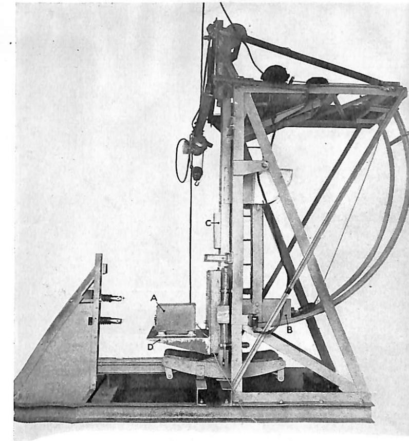
*Light-weight shock-testing machine at N.R.L. The equipment under test is shown at A, mounted on fixture which is attached to the anvil plate. B and C are the 400-pound horizontal and vertical hammers.*
