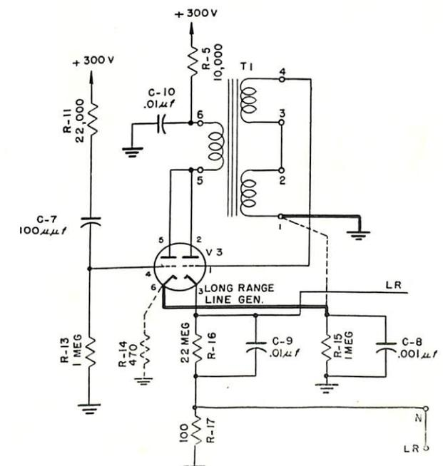
Circuit changes for increased long-range line brilliance. Added wires are shown heavy, and dashed lines indicate wires removed.
