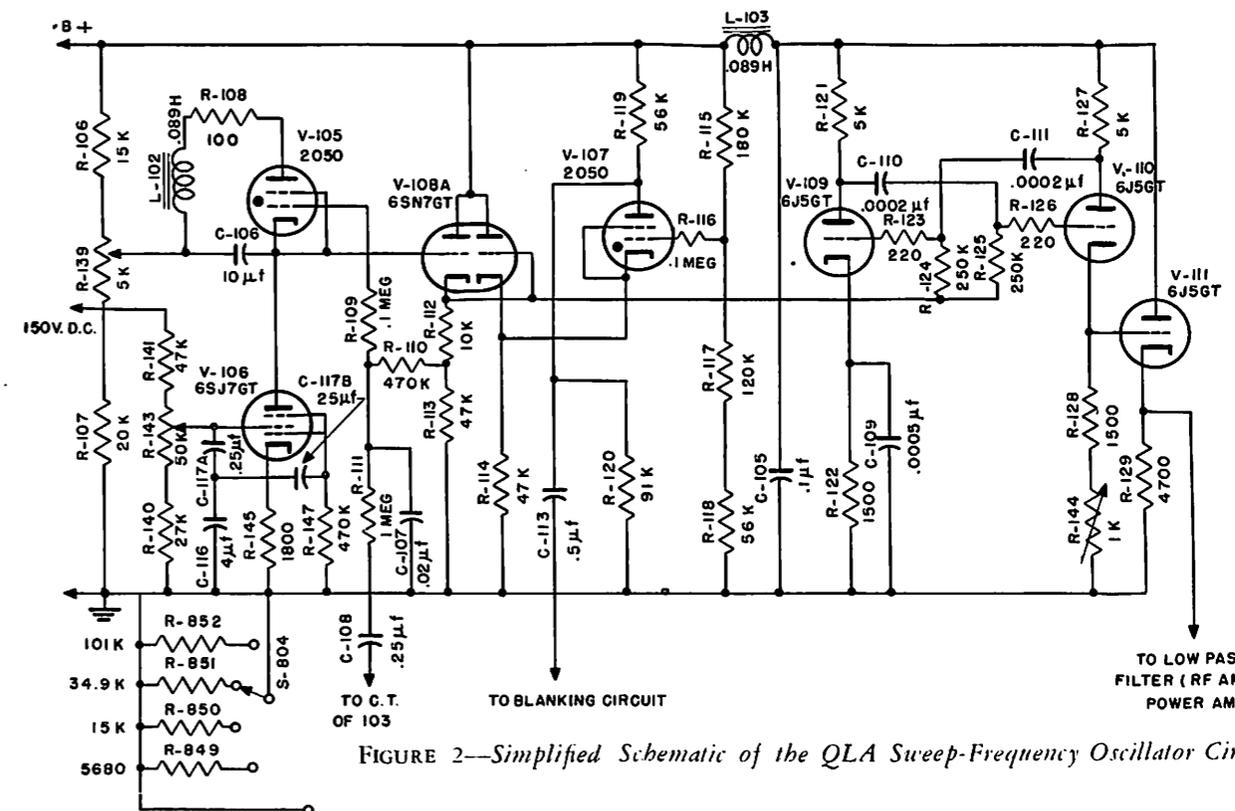
FIGURE 2—Simplified Schematic of the QLA Sweep-Frequency Oscillator Circuits
