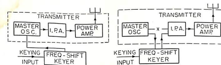
FIGURE 5.—Two arrangements for frequency-shift keying a transmitter.
