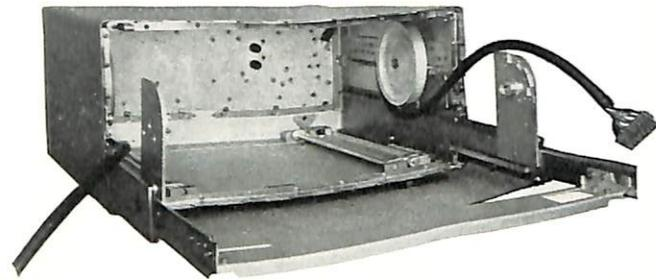
Front view of the RDZ cabinet with chassis-panel assembly removed to show details of the slide mechanism and cable take-up wheels. The cable filter assembly is shown in position at the rear of the cabinet.
