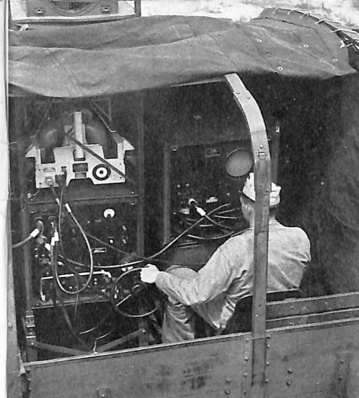
The 1B mounted in a USMC 6x6 truck, showing position of operator and equipment.
