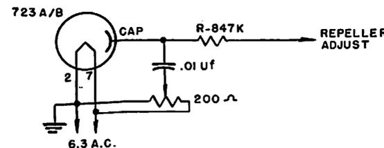
plest AFC," consists of superimposing a small amount of 60-cycle voltage on the repeller of the local oscillator, thereby swinging the frequency of the L.O. It was found that the tuning was more stable and that varying the length of the periscope adapter did not cause the echoes to disappear as they had formerly. As might be suspected, the echoes will be lacy if too much ac is used, but it was found that adding 1.5 to 2 volts gave good results.
