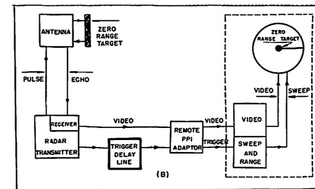
Block diagram showing location of the delay line to compensate for fixed range-error.
