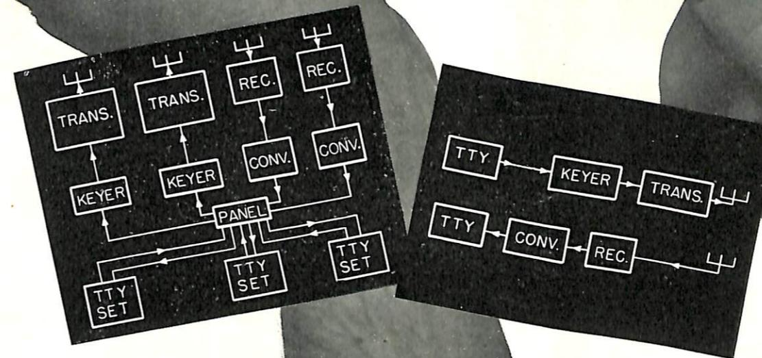
Typical large-ship installation includes a transfer panel to permit independent use of all units.
