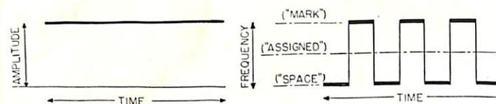
FIGURE 4.—Receiver response to FSK telegraph signals converted by (left) a conventional detector and (right) by an FSK receiver-converter.
