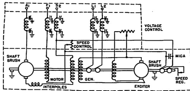
FIGURE 5—A more elaborate filtering system for motor-generators includes shaft-grounding brushes and a capacitor across the speed-regulator contacts as shown.
