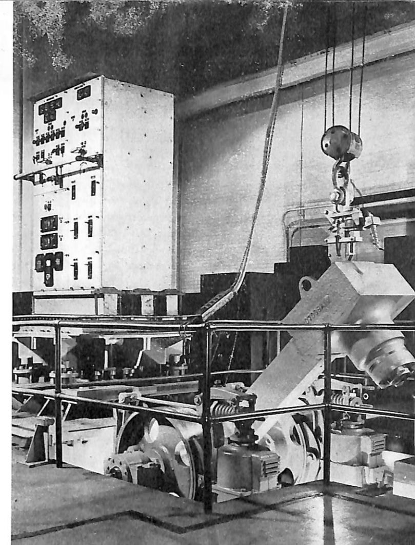
*The medium-weight shock-testing machine at Westinghouse. When released, the hammer starts downward, then swings upwards to strike the anvil plate from beneath.*
