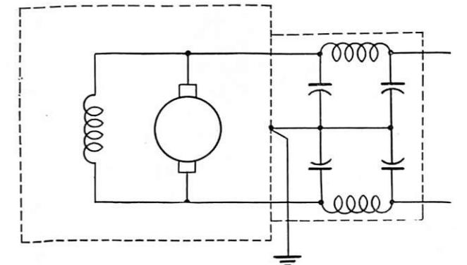
FIGURE 2—More effective interference suppression is obtained with this inductance-capacitance filter.
