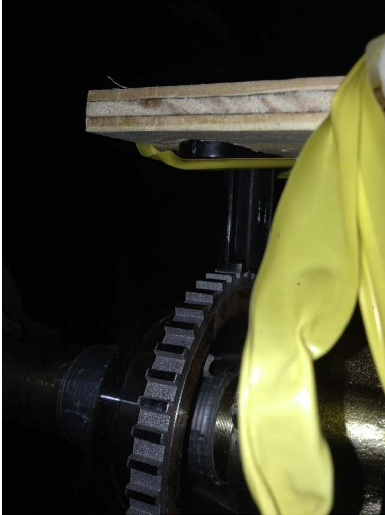
Figure. Wheel speed sensor hack.
