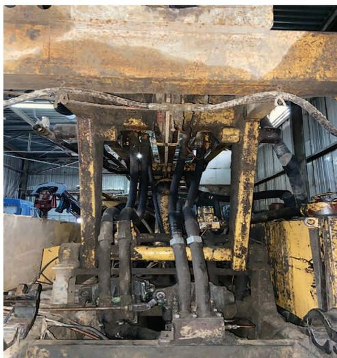
*Fig. 1. High-pressure hoses of the drilling rig URB-2A2*
